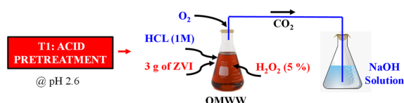
Fig. 2 Simplified illustration of fenton reactions with ZVI oxidation reactor (T2)
