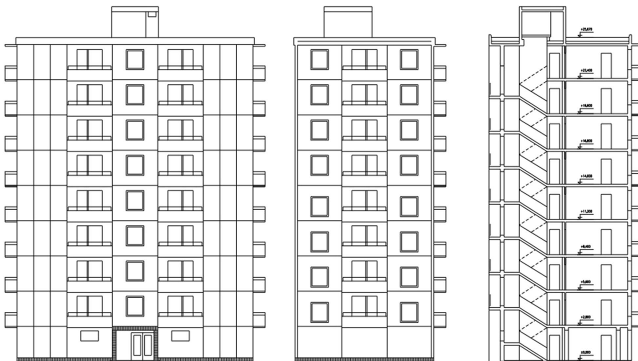
Fig. 4 Architectural section drawings of apartment building type B: front view (left), side view (centre) and cross-section in side view (right)
