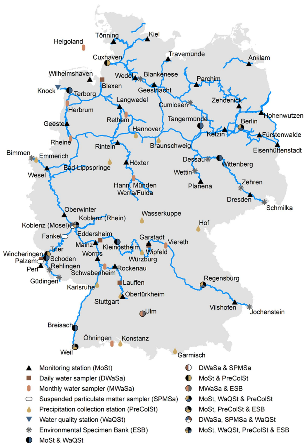
Fig. 5 Monitoring network of the BfG department G4 for environmental radioactivity and qualitative aquatic monitoring
