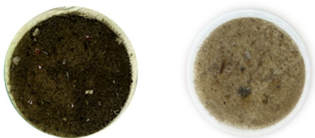
Fig. 1 Whatmann filter with (right) and without (left) pre-treatment with Fenton's reagent
